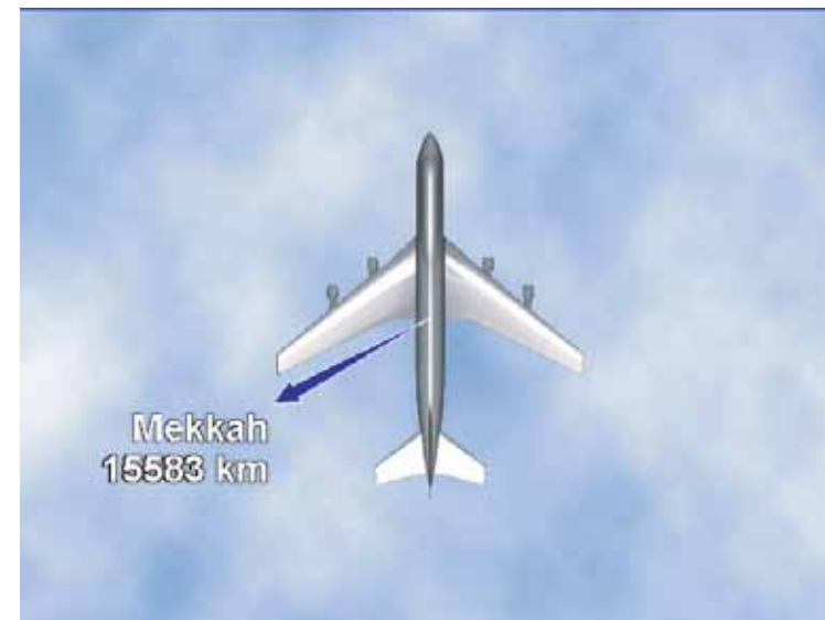
Distance & direction indicator provides information relative to current aircraft position. Aircraft icon, background image, style & color are all user-configurable
